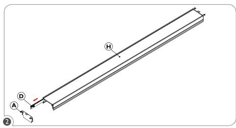
Remove one end plate (A) from the optical engine (H) and slide LED boards (D) out of the side channel. Disconnect quick connectors and re-connect all new boards. Make sure they have proper orientation - with LED row aligned with LED's on adjacent boards. Slide boards back in the side channel and re-attach the end plate.
