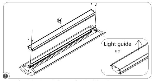
Re-attach optical engine (H) in the same orientation (light guide up).
