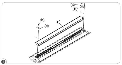
Remove top cover retaining screws (B) with a screwdriver and remove top covers (C) and optical engine (H).
