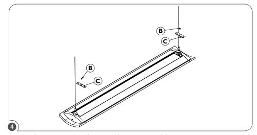
Re-attach top covers (C) and secure with top cover retaining screws (B).
