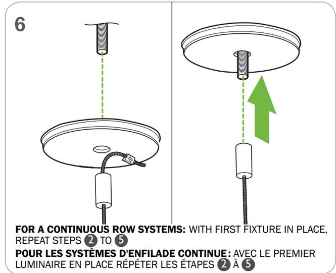
**FOR A CONTINUOUS ROW SYSTEMS: WITH FIRST FIXTURE IN PLACE, REPEAT STEPS 2 TO 5**
