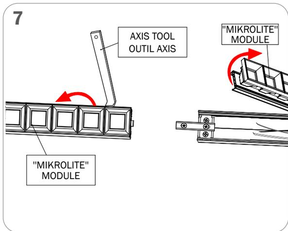
PULL AWAY MIKROLITE MODULES FROM FIXTURES TO GET ACCESS TO QUICK-WIRE CONNECTIONS
