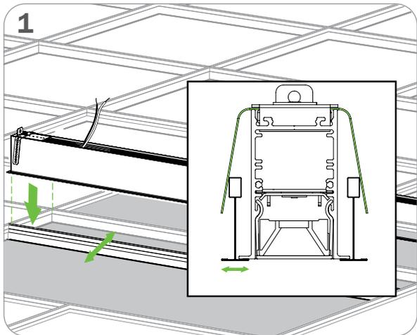
ADJUST T-BAR RUNNER TO THE FIXTURE WIDTH
