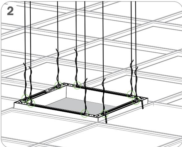
SECURE SUPPORT WIRES TO THE FIXTURE
