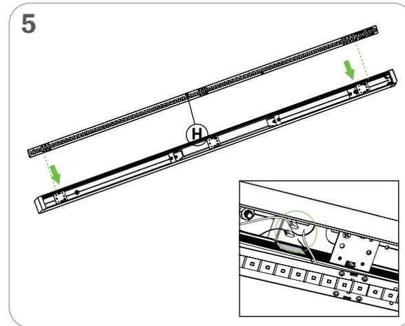
MAKE SURE THAT MODULE BRACKET IS WELL SNAPPED INTO PLACE
