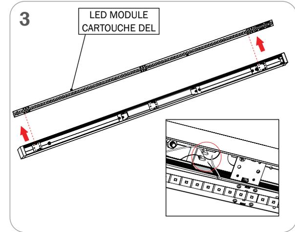
DROP LED MODULE OUT OF THE FIXTURE
