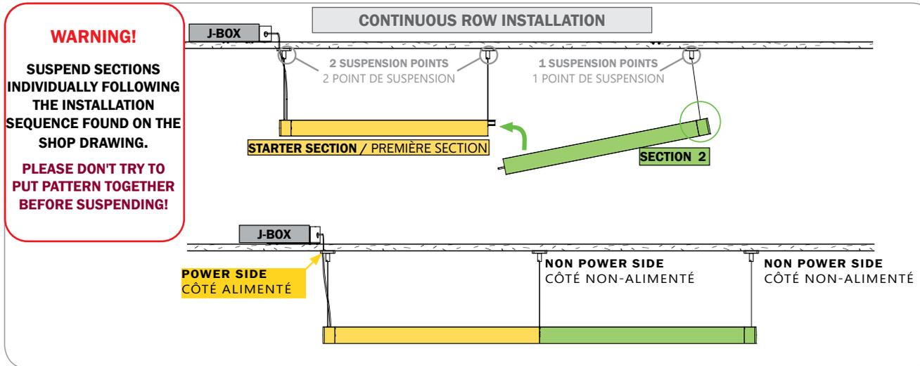
**CONTINUOUS ROW: FOLLOW STEPS 1 TO 3 TO INSTALL NEXT FIXTURE IN CEILING, THEN: REMOVE COVERS.**
