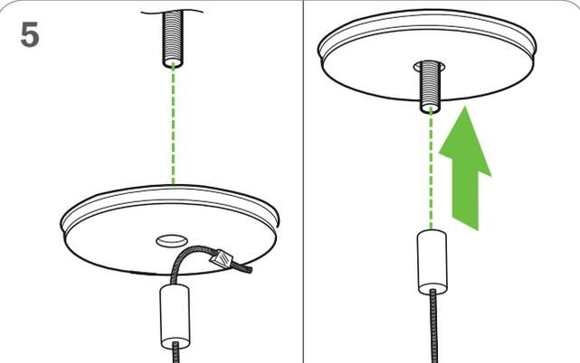
**FOR A CONTINUOUS ROW SYSTEMS: WITH FIRST FIXTURE IN PLACE, REPEAT STEPS 2 AND 4, PLACE CANOPY ON THREADED STUD AND FEED THE AIRCRAFT CABLE FOR THE NEXT FIXTURE IN LINE.
