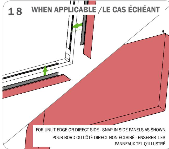
FOR UNLIT EDGE OR DIRECT SIDE - SNAP IN SIDE PANELS AS SHOWN
