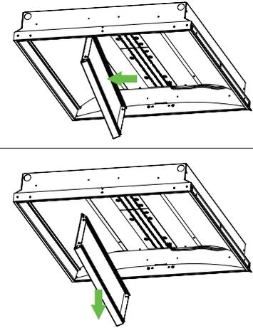
MOVE LENS SIDWAYS UNTIL LENS CAN BE LOWERED WITHOUT HITTING HOUSING.
