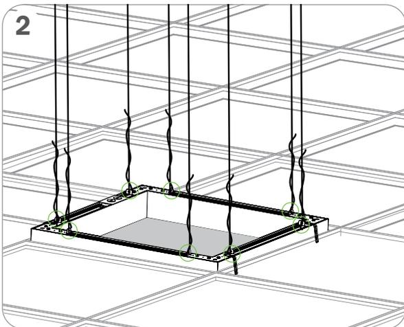
SECURE SUPPORT WIRES TO THE FIXTURE
