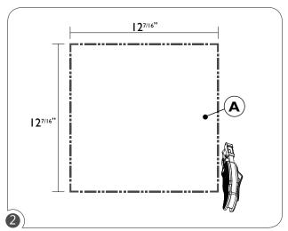
Cut the tile (A) with a utility knife according to the diagram and measurement located above. Make sure that the hole is centered and square.
