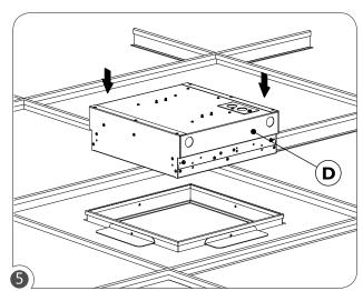
Insert the fixture (D) into the frame. Ensure that the fixture is correctly oriented in relation to other fixtures.
