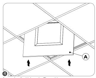
Insert the tile (A) into the Tbar grid.
