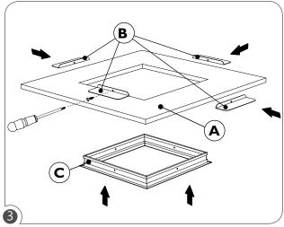
Insert the drywall flange into the hole and fix into place with the 4 brackets (B) and screws. Make sure that the drywall kit (C) is tight against the tile (A).
