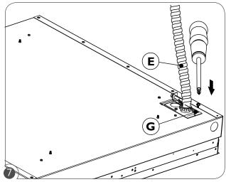
Push connected wires and wire nuts into fixture. Reinstall knockout plate (G) onto fixture by hooking tab into hole, and refastening screw to knockout plate and housing.
