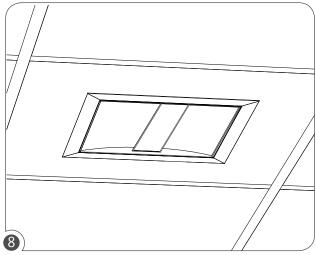
Test the fixture to ensure proper connections. Re-install the remaining tile to close the ceiling.
