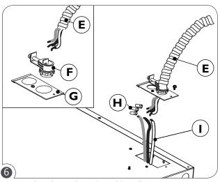
Remove knockout plate (G) and install BX connector (F) through the knockout plate (G). Insert BX cable (E) into BX connector (F).
