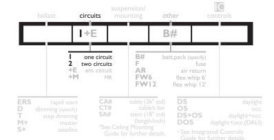
In the Custom Description box on the spec sheet, please specify ALTERNATING or LEFT-RIGHT arrangement for dual circuit
