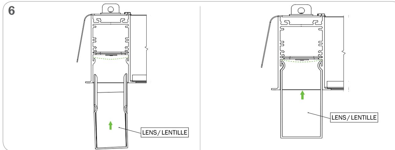
PUSH THE NEW LENS INSIDE AND PRESS ON THE WHOLE LENGTH TO INSERT
