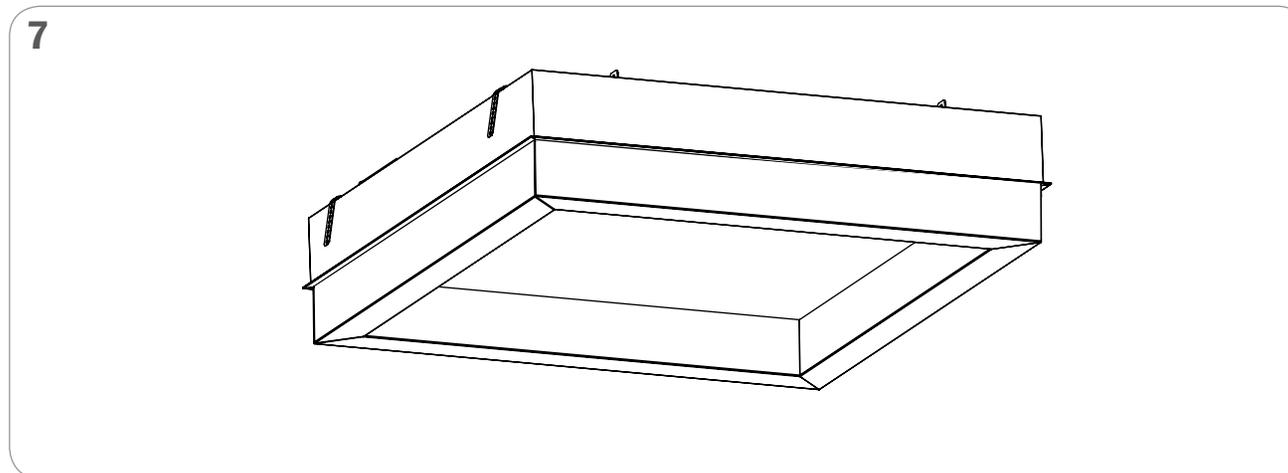
MAKE SURE THAT THE LENS IS FIRMLY SEATED AND LEVELLED ALONG THE WHOLE LENGTH OF THE FIXTURE
