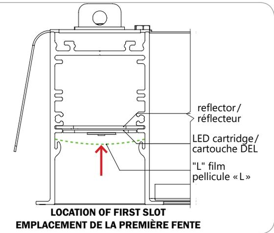
**INSTALL "L" FILM IN ALL CORNERS (4 FOR EACH FIXTURE)** SLIDE THE "L" FILM INTO ONE EXTRUSION'S END INTO THE FIRST SLOT
