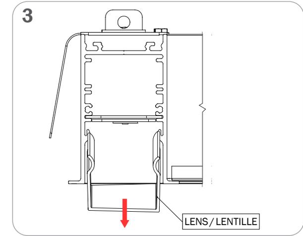
MOVE THE TOOL OVER TO ONE SIDE TO PREVENT LENS FROM BREAKING
