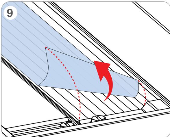
Remove the film from lens only **AFTER** sanding and
