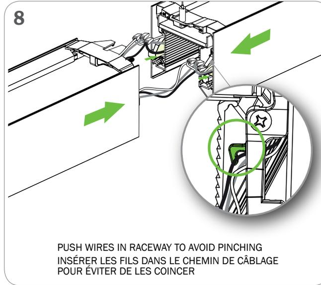
PUSH WIRES IN RACEWAY TO AVOID PINCHING
