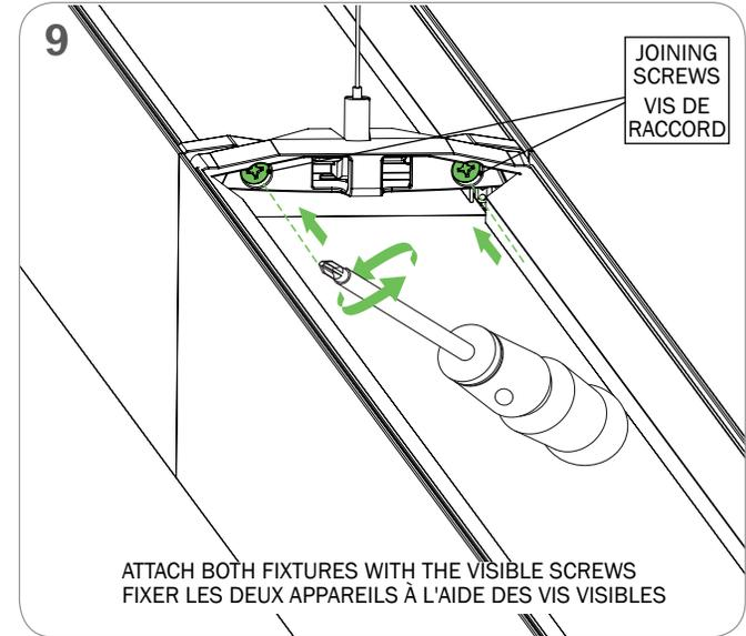
ATTACH BOTH FIXTURES WITH THE VISIBLE SCREWS
