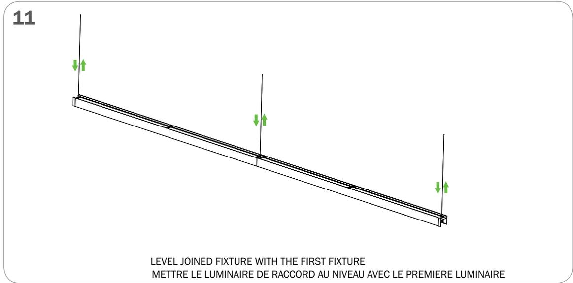
LEVEL JOINED FIXTURE WITH THE FIRST FIXTURE
