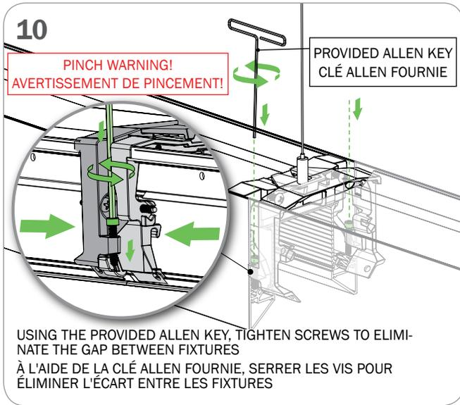
USING THE PROVIDED ALLEN KEY, TIGHTEN SCREWS TO ELIMINATE THE GAP BETWEEN FIXTURES
