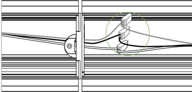
CONNECT WIRES AND REINSTALL REMOVED OPTICS
