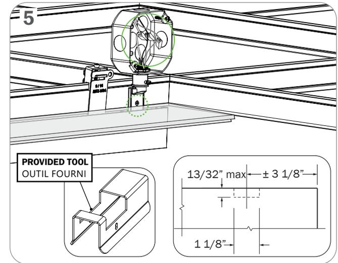
**NOTCH CEILING TILE. USE PROVIDED TOOL. PLEASE REFER TO DIAGRAM FOR NOTCH SIZE AND PLACEMENT**
