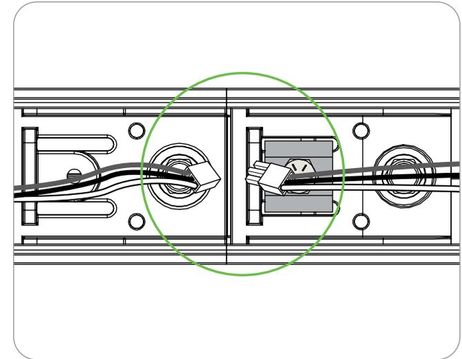
**MAKE ELECTRICAL CONNECTIONS BETWEEN SEGMENTS IN MULTIPLE CIRCUIT RUNS, PLEASE REFER TO LABELS ON CONNECTORS FOR APPROPRIATE PAIRINGS.**
