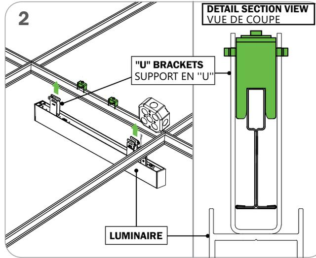
**INSERT LUMINAIRE ON T-BAR BY USING "U" BRACKETS**
