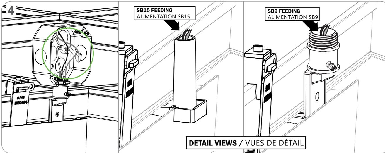
**CONNECT FIXTURE WIRES TO JUNCTION BOX / CONNECTEZ LE LUMINAIRE À LA BOÎTE DE JONCTION**
