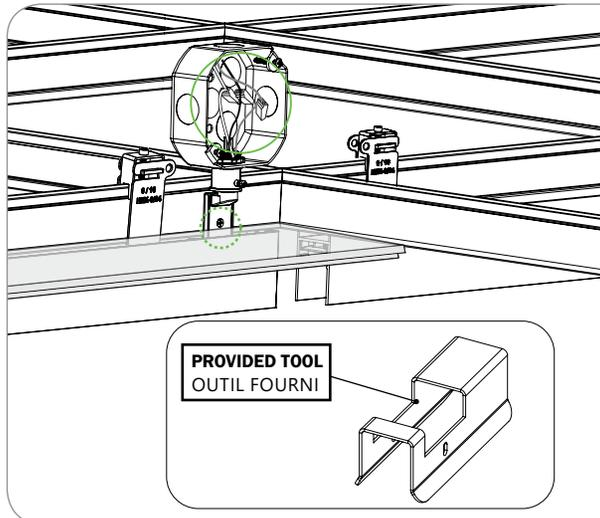
**NOTCH CEILING TILE. USE PROVIDED TOOL. PLEASE REFER TO DIAGRAM FOR NOTCH SIZE AND PLACEMENT**
