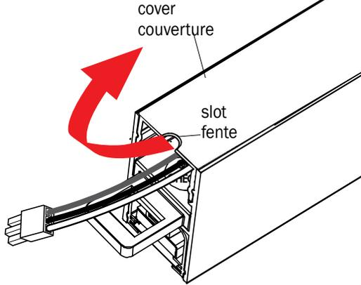
CONTINUOUS ROW: FOLLOW STEPS 1 TO 3 TO INSTALL NEXT FIXTURE IN CEILING, THEN: REMOVE COVERS.
