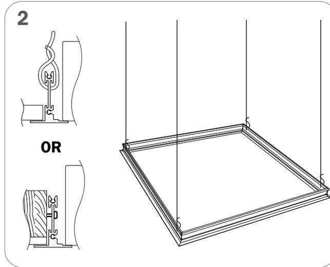
INSERT THE DRYWALL KIT INTO THE HOLE AND ATTACH IT TO A WOODEN FRAME USING WOOD SCREWS **OR** HANG IT USING HANGER WIRES
