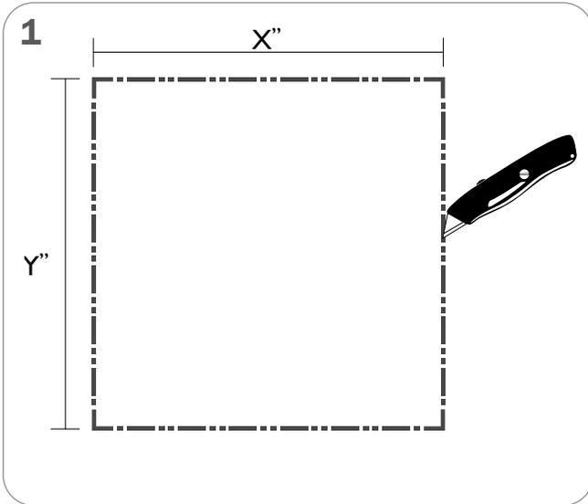
1 MAKE AN OPENING IN DRYWALL ACCORDING TO THE DIMENSIONS ON THE SHOP DRAWINGS
