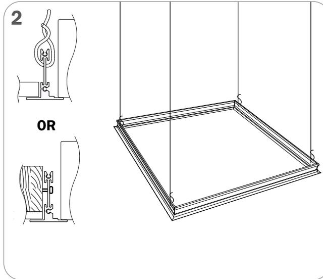
2 INSERT THE DRYWALL KIT INTO THE HOLE AND ATTACH IT TO A WOODEN FRAME USING WOOD SCREWS **OR** HANG IT USING HANGER WIRES
