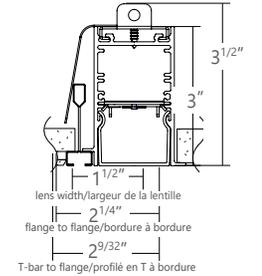
**MFST** MiniFlange SCREW SLOT T-BAR
