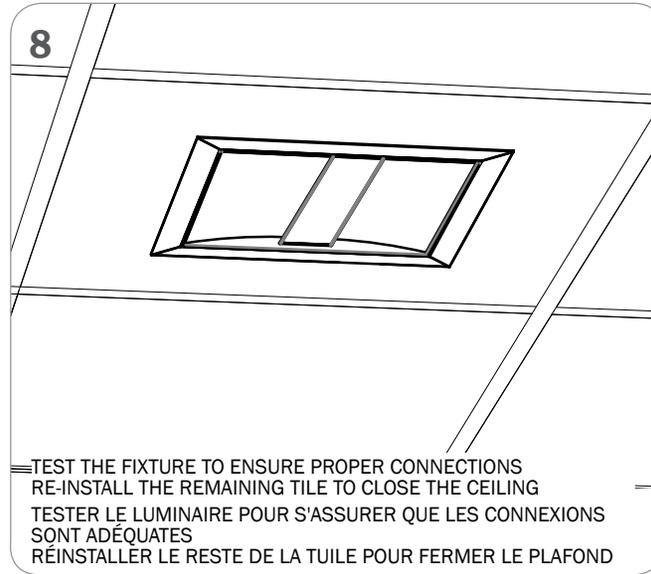
TEST THE FIXTURE TO ENSURE PROPER CONNECTIONS
