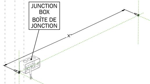
LOCATE THE MOUNTING POINTS ON THE WALL. MAKE HOLES AND USE DRYWALL ANCHORS IF ANY OF THE HOLES DO NOT LINE UP WITH A STRUCTURAL STUD. LOCATE POSITION OF THE JUNCTION BOX ON THE WALL. REPÉRER LES POINTS DE MONTAGE SUR LE MUR. PERCER LES TROUS ET UTILISER LES ANCRAGES DE GYPSE SI UN DES TROUS N'EST PAS ALIGNÉ AVEC UNE SOLIVE DE LA STRUCTURE. REPÉRER LA POSITION DE LA BOÎTE DE JONCTION SUR LE MUR.
