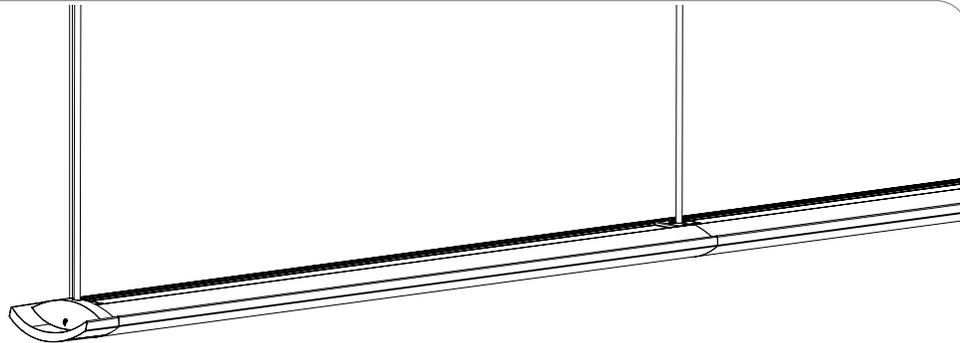
**FOR A CONTINUOUS ROW SYSTEMS:** WITH FIRST FIXTURE IN PLACE, REPEAT STEPS 1 TO 4 FOR THE NEXT FIXTURE IN LINE
