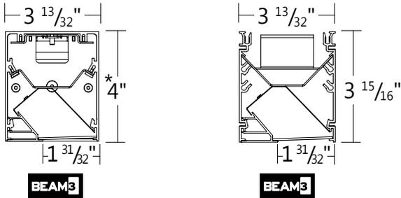
\* 4" for flush fixtures and 4 3/4" for regressed fixtures
