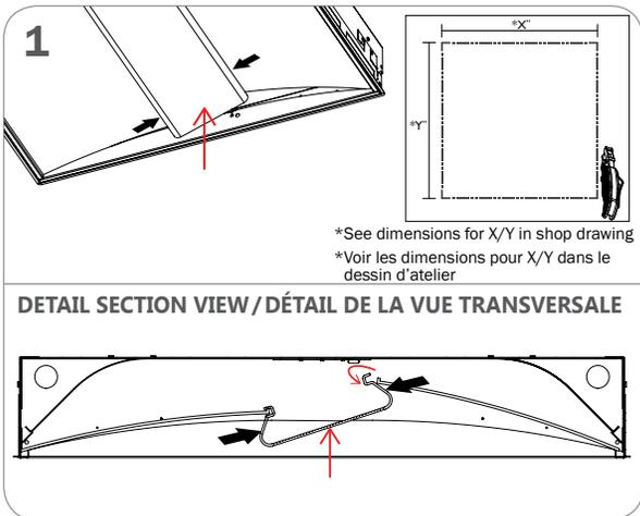
SQUEEZE LIGHTLY ON CENTER LENS SIDES WHILE PUSHING UP SLIGHTLY AND ROTATING LENS UNTIL ONE SIDE OF LENS IS FREE, THEN LOWER. PULL ON SIDE LENS TO REMOVE OPTICAL ENTIRELY FROM FIXTURE.
