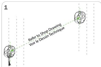
Ensure that the power to the fixture's circuit is turned off. Locate position of the junction box on the wall.
