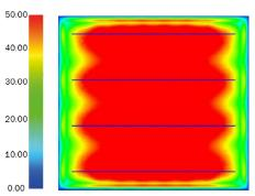
Average light levels: 50 fc Power density: 0.52 W/ft2 750 lm/ft, 16' on center 9.5' ceiling, Max/Min 2.88, Avg/Min 2.04
