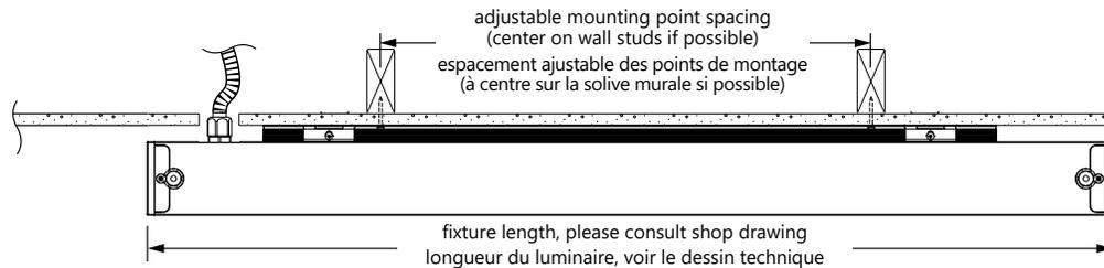
**1** **NOTE:** 9" MINIMUM CLEARANCE SPACE IS NEEDED AT THE TOP OF THE FIXTURE. TOP OF THE RAIL ALIGNS WITH TOP OF THE FIXTURE.
