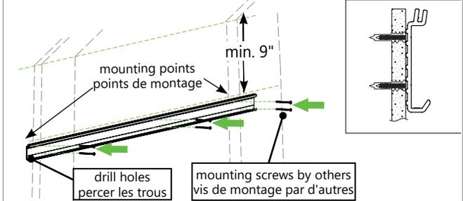
INSTALL WALL RAIL TO WALL USING WALL ANCHORS (BY OTHERS). START RAIL AT 4" FROM END OF FIXTURE.
