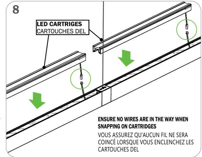
**MAKE ELECTRICAL CONNECTIONS IN MULTIPLE CIRCUIT RUNS, PLEASE REFER TO LABELS ON CONNECTORS FOR APPROPRIATE PAIRINGS**
