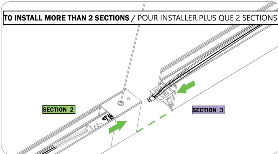
**FOLLOW STEPS 4-6 FOR EACH ADDITIONNAL SECTION. WHEN RUN IS ALL MOUNTED, PROCEED WITH STEPS 7 AND 8 TO COMPLETE INSTALLATION.**
