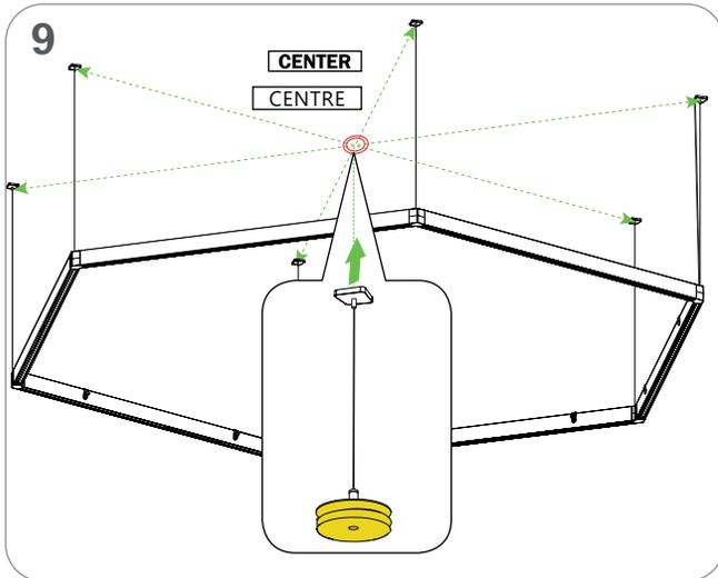
**FIND HEXAGON CENTER AS PER SHOP DRAWING DIMENSIONS AND INSTALL PANEL SUPPORT CAROUSEL**
