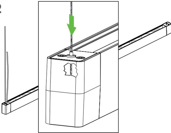
**HANG 1ST SECTION IN RUN BY THREADING SUSPENSION CABLES THROUGH GRIP LOCKS AS SHOWN.**
