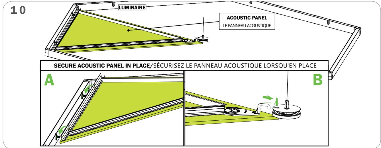
**SECURE ACOUSTIC PANEL IN PLACE / SÉCURISEZ LE PANNEAU ACOUSTIQUE LORSQU'EN PLACE**
