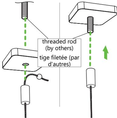
**PLACE CANOPIES IN POSITION ACCORDING TO THE SHOP DRAWING. HANG SUSPENSION CABLES.**
