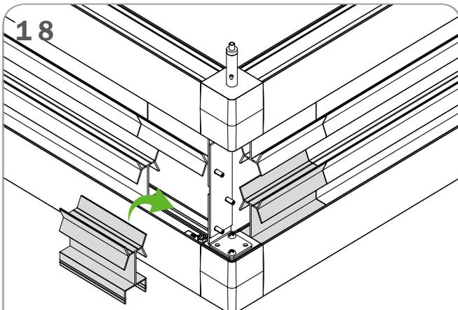
MAKE SURE TO REINSTALL ALL OF THE REMOVED SIDE EXTRUSION PIECES ONCE ALL THE BOTTOM FRAMES ARE ASSEMBLED AND WIRED
