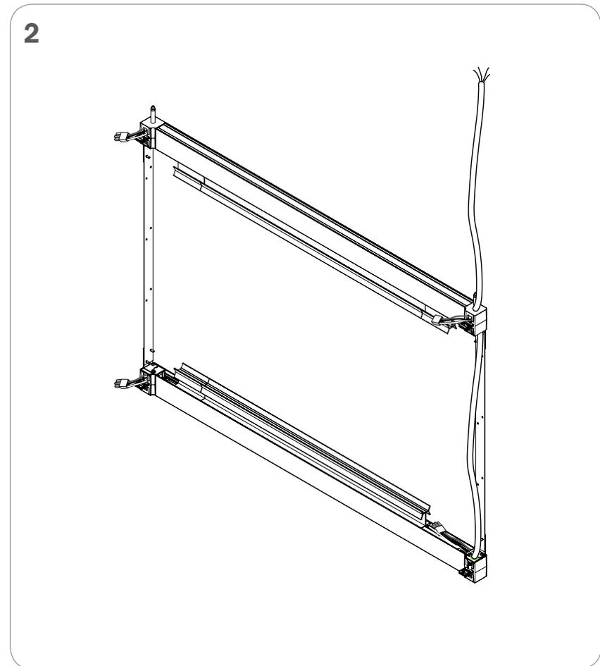
ASSEMBLE SECTION 1 AND 5 WITH SUPPORT PLATES
