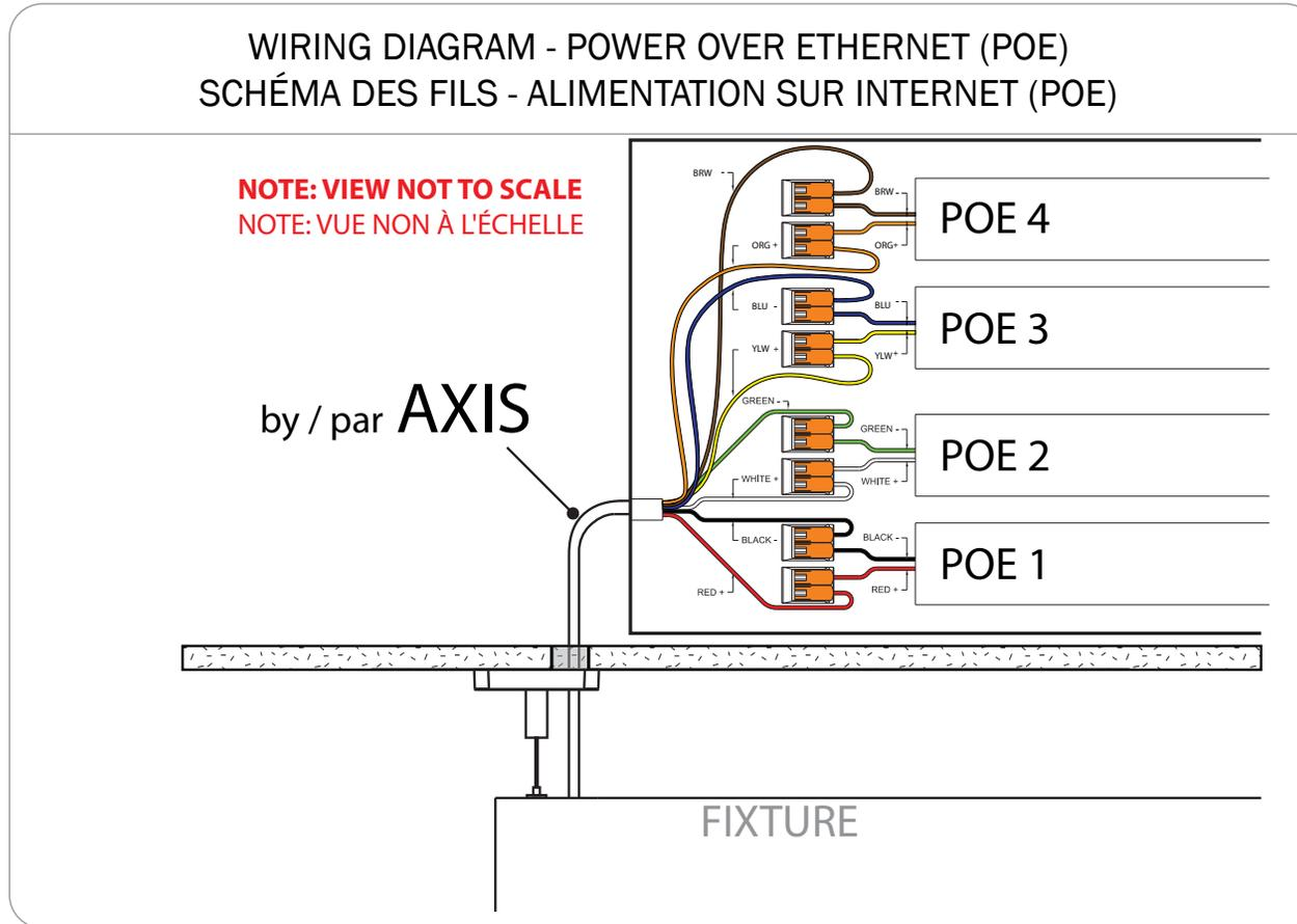
**RUN POWER CABLE FROM FIXTURE THROUGH CEILING AND UP TO THE DRIVER BOX. MAKE CONNECTIONS ACCORDING TO WIRING DIAGRAM.**
