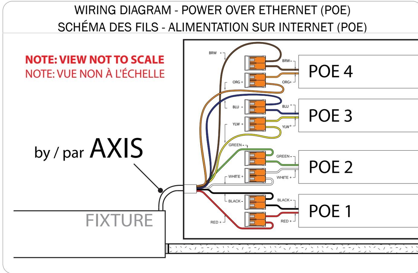
**RUN POWER CABLE FROM FIXTURE THROUGH CEILING AND UP TO THE DRIVER BOX. MAKE CONNECTIONS ACCORDING TO WIRING DIAGRAM.**
