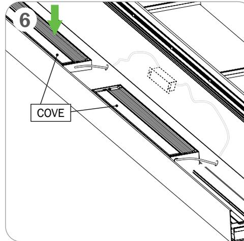
**CONTINUOUS ROW:** CONNECT CABLE OF EACH FIXTURE TO POE SWITCH
