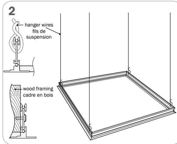
INSERT THE DRYWALL KIT INTO THE HOLE AND ATTACH IT TO A WOODEN FRAME OR HANG IT USING HANGER WIRES. MAKE SURE THAT THE FRAME IS TIGHT AGAINST THE CEILING.
