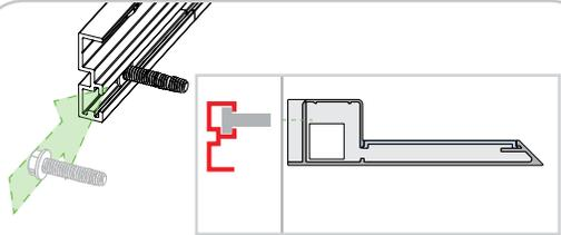
INSTALL FIXTURE MOUNTING SCREWS BY SLIDING THEM INTO THE TRACK PRIOR TO MOUNTING THE TRACK (SEE STEP 1) AND ADDING THE TRACK END CAPS. /
